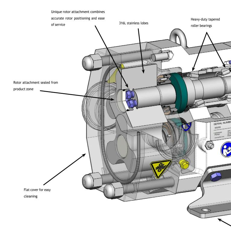
Easy access to shims for rotor clearance adjustment
